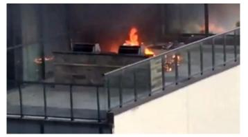
Wind-driven fires are more problematic in high-rise buildings as wind speed increases with height. They are recognizable by smoke exiting windows with the hallway acting as a fireplace chimney. High-rise fires must be fought indoors rather than from a distance while evacuating hundreds or thousands of residents. Open doors make fires more dangerous.
